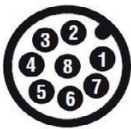
(Connector) M12x1; 8-pole, A-coded
