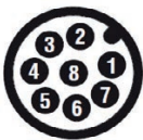
(Connector) M12x1; 8-pole, A-coded
